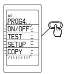
You can check the timer program setting by transmitting the Timer Macro signals.
